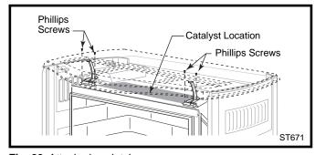
Fig. 20 Attach glass latches.
